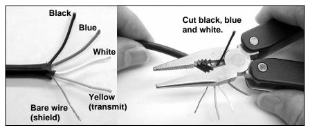
After removing the adapter segment, prepare to connect by removing and taping off unneeded wires. Strip the end of the yellow wire.
